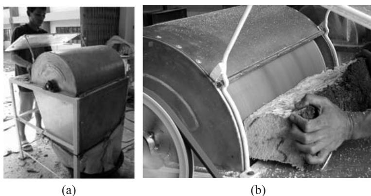
**Fig. 2.** Prototype of the developed sago-pith grating machine (a) and the grater blade during operation (b).
