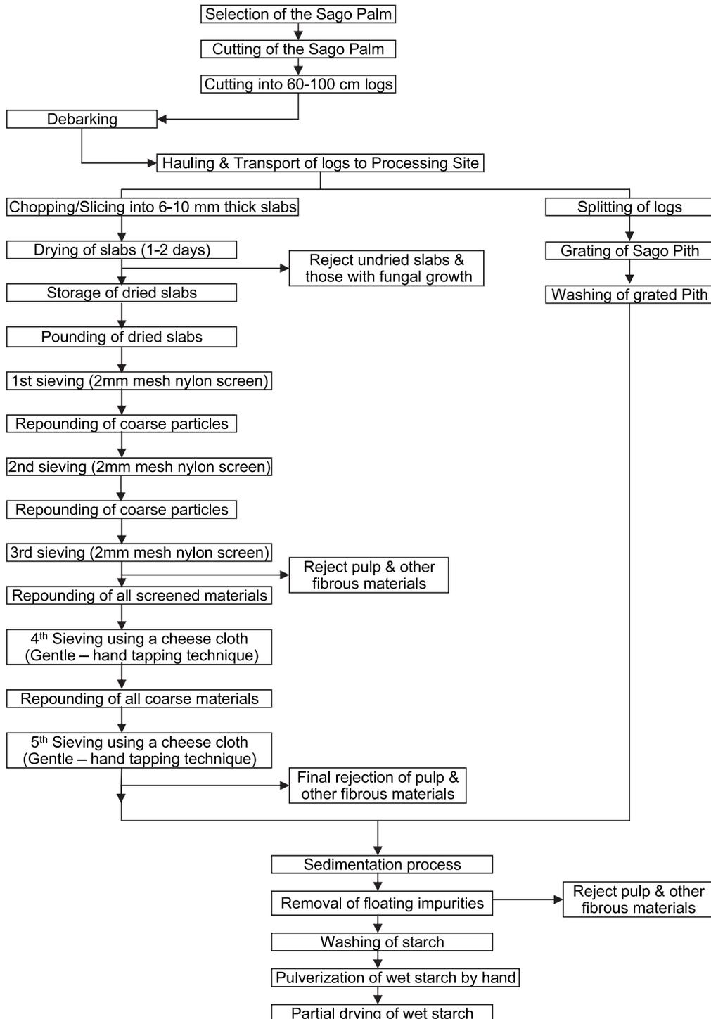
**Fig. 1.** Flowchart showing the traditional starch processing (left column) in the Philippines and the improved method (right column) with the developed grating machine. (Loreto and Quevedo, 2004).
